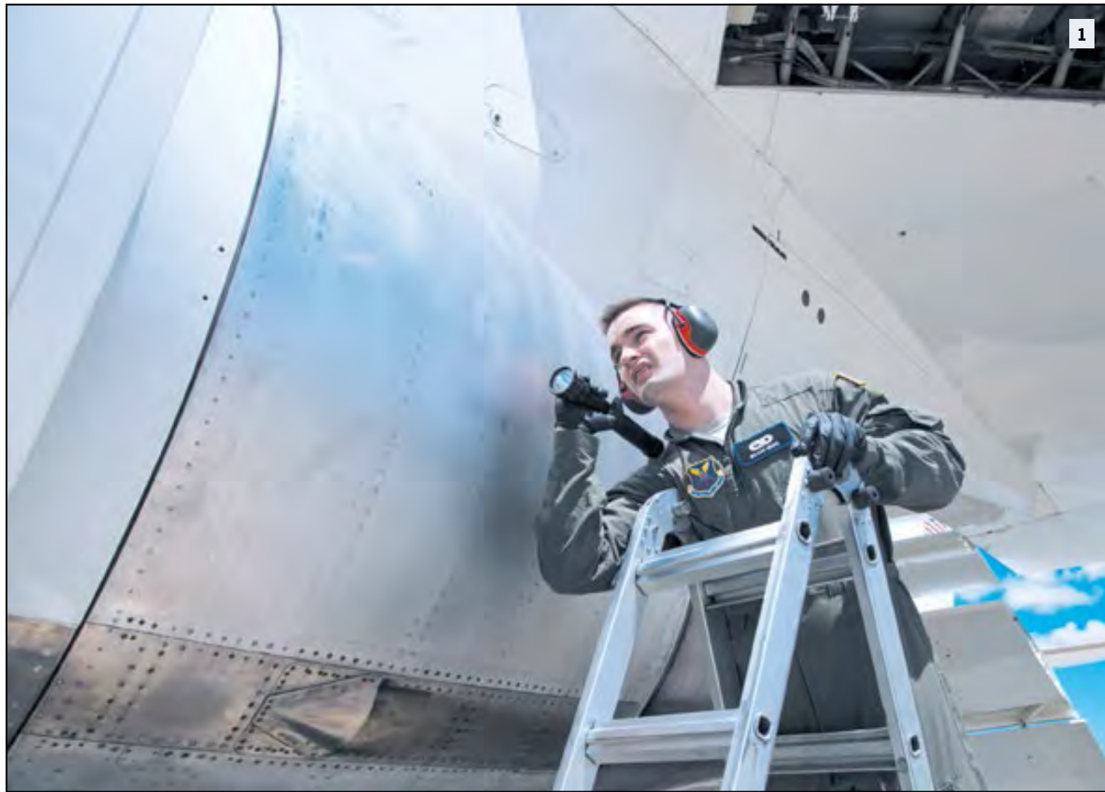
1) Senior Airman Cody Grauel, 595 Aircraft Maintenance Squadron propulsion journeyman, inspects the engine of an E-4B for any damage or leaks after arriving June 9 at Travis Air Force Base, Calif. The E-4B, from Global Strike Command, Barksdale Air Force Base, La., provides support to the Federal Emergency Management Agency, which provides communications and command center capability to relief efforts following natural disasters, such as hurricanes and earthquakes.
